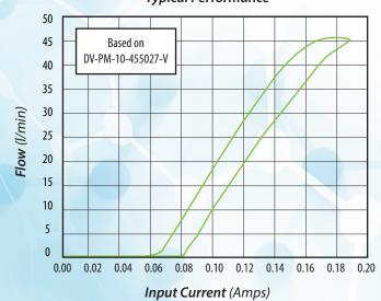
The above flow curve is a typical calibration record for the DVP. All proportional valves have a stored calibration data sheet readily available upon request.
