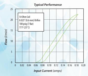
The above flow curve is a typical calibration record for the EVP. All proportional valves have a stored calibration data sheet readily available upon request.
